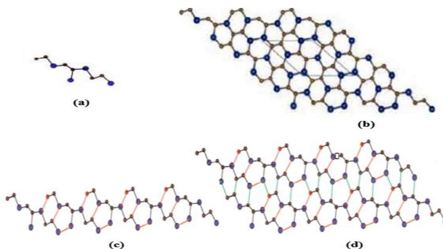
Figure 3. Two Dimensional structure of  $(Si_2C_3 - II[p, q])$  with carbon (brown) and silicon (blue). a) One dimensional unit cell of  $(Si_2C_3 - II[p, q])$ . b) Structure of  $(Si_2C_3 - II[3,3])$ . c) Structure of  $(Si_2C_3 - II[5,1])$ . d) Structure of  $(Si_2C_3 - II[5,2])$ .
