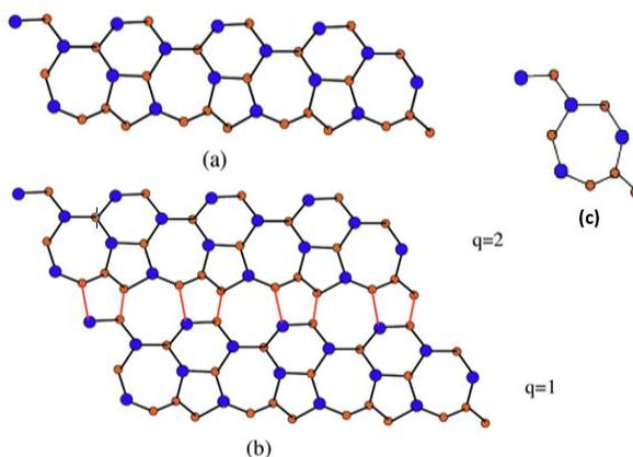
Figure 1. Two Dimensional structure of  $(Si_2C_3 - I[p, q])$  with carbon (brown) and silicon (blue). a).  $(Si_2C_3 - I[4,1])$  one row with  $p=4$  and  $q=1$ . b)  $(Si_2C_3 - I[4,2])$ . c)  $(Si_2C_3 - I[1,1])$ .
