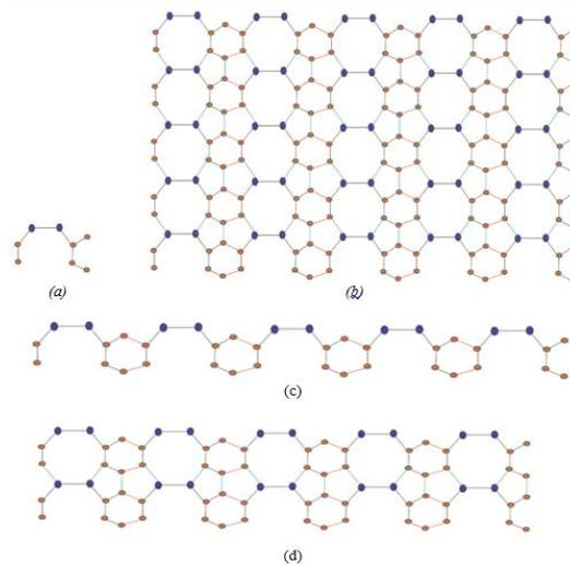
Figure 7. Two Dimensional structure of  $(SiC_3 - III[p, q])$  with carbon (brown) and silicon (blue). a) One dimensional unit cell of  $(SiC_3 - III[p, q])$ . b) Structure of  $(SiC_3 - III[5,5])$ . c) Structure of  $(SiC_3 - III[5,1])$ . d) Structure of  $(SiC_3 - III[5,2])$ .
