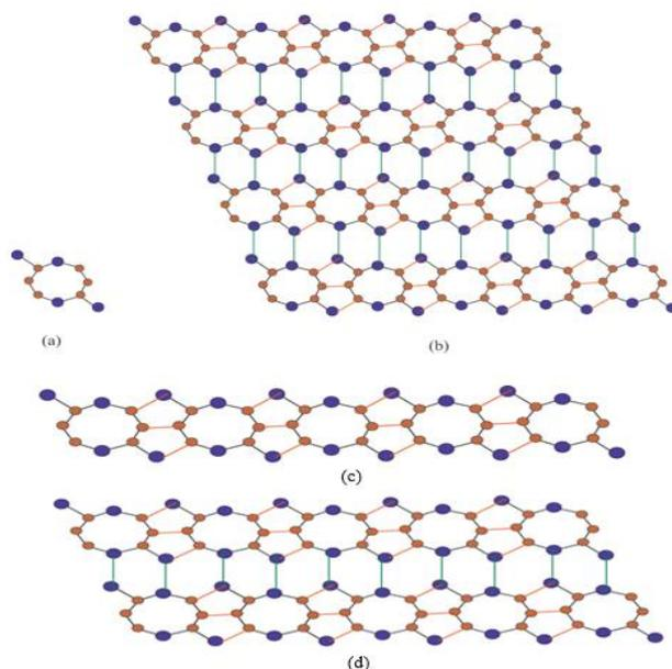
Figure 5. Two Dimensional structure of  $(Si_2C_3 - III[p, q])$  with carbon (brown) and silicon (blue). a) One dimensional unit cell of  $(Si_2C_3 - III[p, q])$ . b) Structure of  $(Si_2C_3 - III[5,4])$ . c) Structure of  $(Si_2C_3 - III[5,1])$ . d) Structure of  $(Si_2C_3 - III[5,2])$ .
